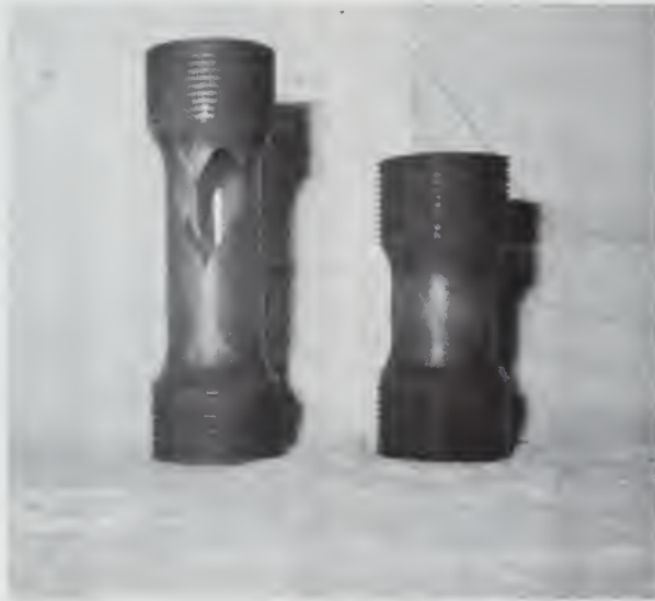
FIGURE 14. FAILED BIAXIAL SPECIMEN. SHOWN LEFT TO RIGHT, FRACTURED BIAXIAL TENSILE SPECIMEN AND YIELDED BIAXIAL COMPRESSIVE SPECIMEN.
